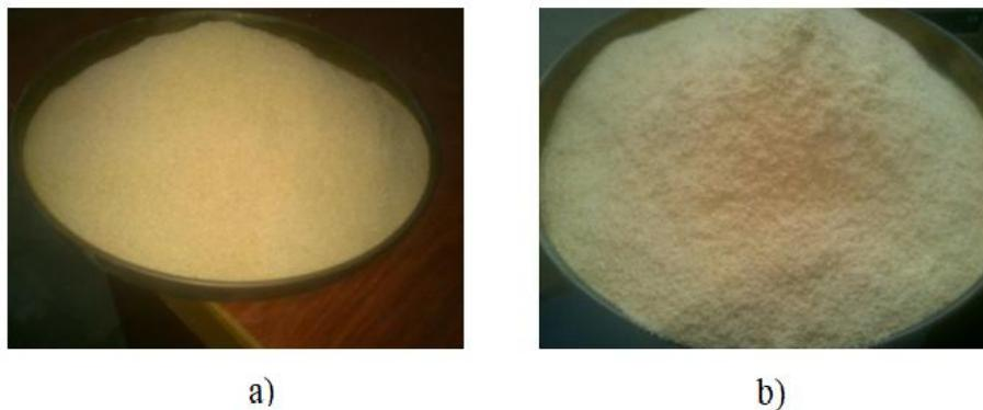
**Figure 3.** Beech wood powder: a) small diameter and b) medium diameter.
