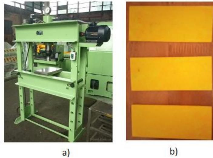
**Figure 4.** a) Semi-hydraulic press and b) samples UPR + organic filler.
