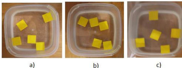
**Figure 5.** Test samples: a) UPR + 150% organic filler, b) UPR + 200% organic filler; and c) UPR + 250% organic filler.
