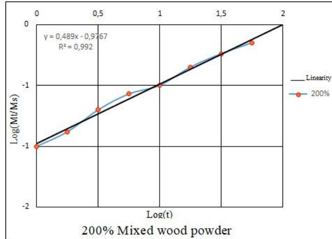
**Figure 10.** Dependency describing the diffusion behavior of samples made from 200% mixed wood powder.
