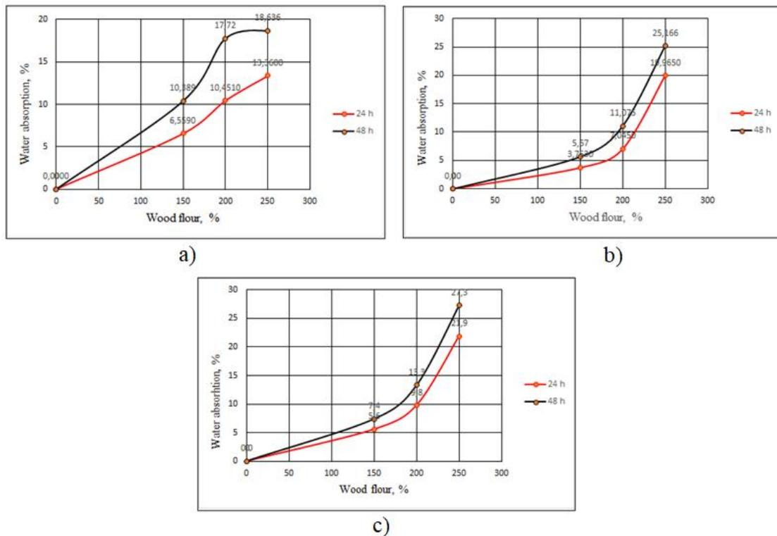
**Figure 7.** Water absorption of polyester samples depending on the percentage content of wood powder: a) mixed, b) with particle diameter of 0.125 mm, and c) with particle diameter of 0.3 mm.
