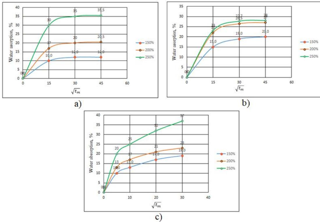
**Figure 9.** Changes in water absorption over time for beech wood powder samples: a) with particle diameter of 0.125 mm, b) mixed, and c) with particle diameter of 0.3 mm.
