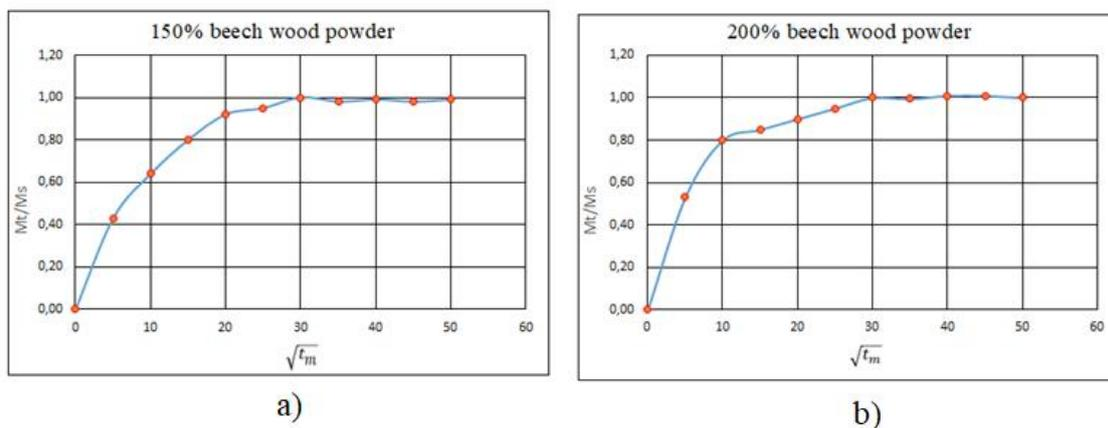
**Figure 11.** Graphs of  $M_t/M_s$  dependence on  $\sqrt{t}$  used for: a) checking the linearity of curves when  $M_t/M_s \leq 0.6$ , and b) deviation from Fickian behavior.
