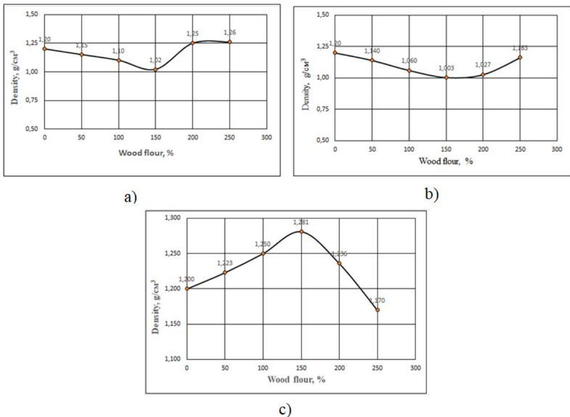
**Figure 6.** Variation in density of unsaturated polyester samples with different content of beech wood powder: a) mixed, b) with particle diameter of 0.3 mm, and c) with particle diameter of 0.125 mm.
