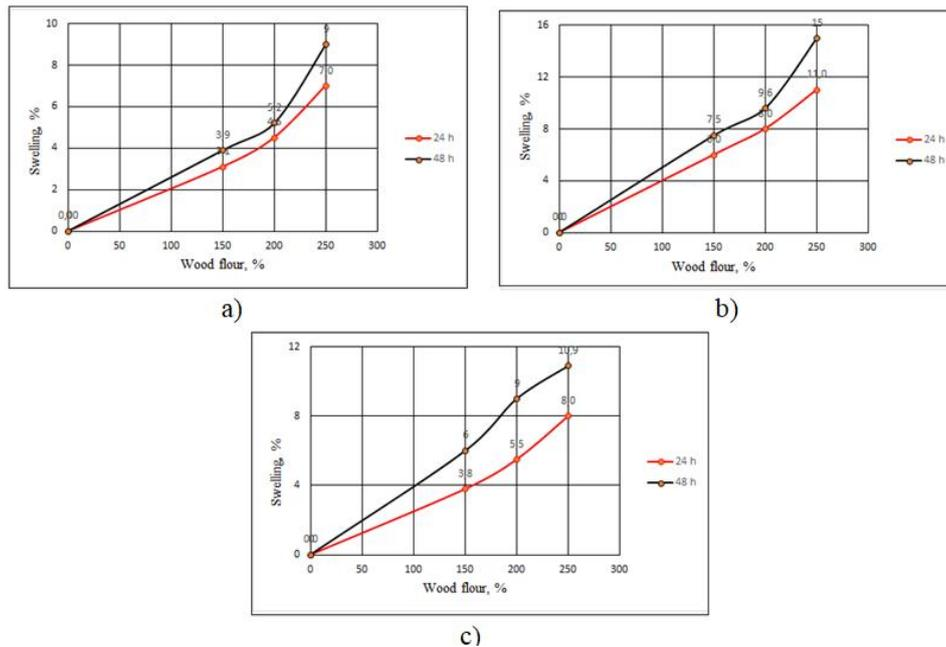
**Figure 8.** Swelling degree of samples in fresh water over a short period with beech wood powder filler of particle diameter: a) 0.125 mm, b) 0.3 mm, and c) mixed.
