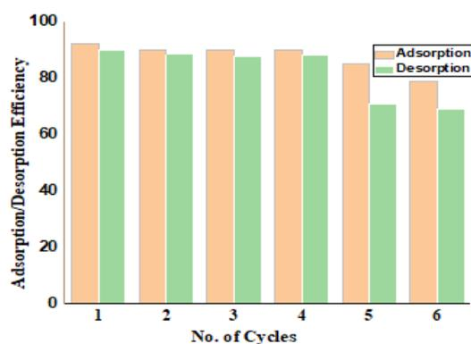
**Figure 9.** Adsorption/Desorption ratios of modified cellulose adsorbent at different cycles.
