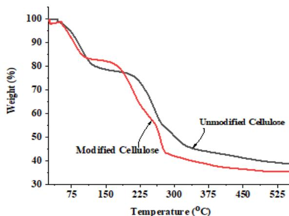
**Figure 3.** The thermograms of unmodified (black) and modified cellulose (red).
