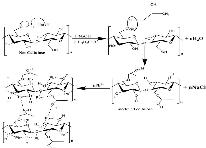
**Figure 2.** Hypothesis representation of Synthesis Schematic and biosorption mechanism of Lead ( $\text{Pb}^{2+}$ ) by modified cellulose<sup>[29–31]</sup>.
