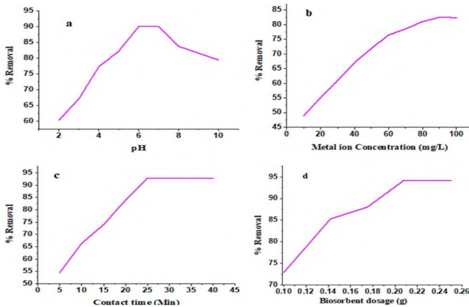
**Figure 5.** Effect of (a) pH, (b) initial ion concentration, (c) contact time, and (d) biosorbent dosage on the adsorption of Pb (II) by the modified cellulose.
