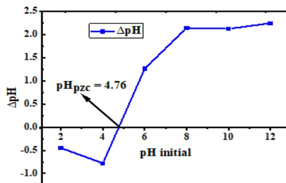
**Figure 6.** Point of zero charge plot of modified cellulose.
