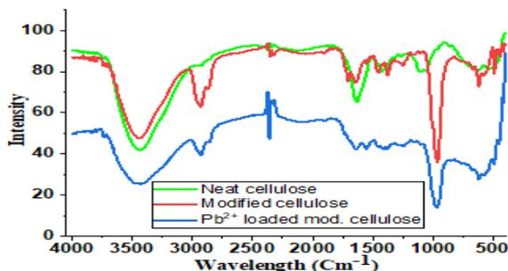
**Figure 1.** FTIR spectra of (green) unmodified cellulose, (red) modified cellulose, (blue) lead ion loaded modified cellulose.
