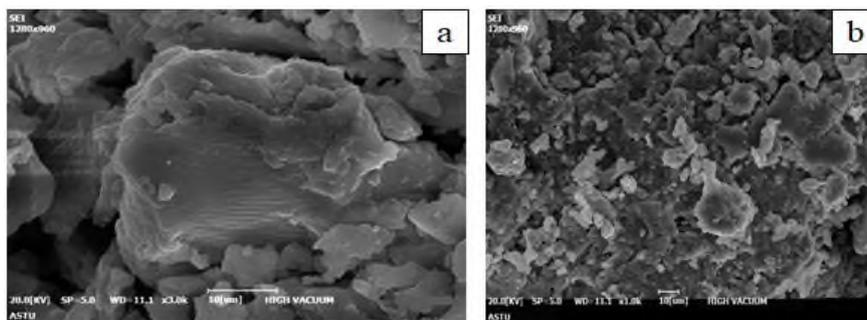
**Figure 4.** SEM image of (a) unmodified cellulose and (b) modified cellulose.
