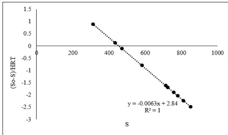
**Figure 5.** The first-order kinetic model for COD removal.
