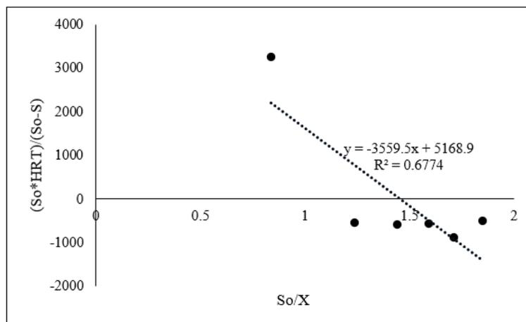
**Figure 6.** The second-order kinetic model for COD removal.
