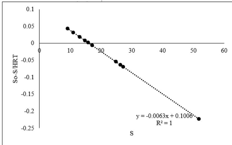
**Figure 8.** The first-order kinetic model for nitrate-N removal.
