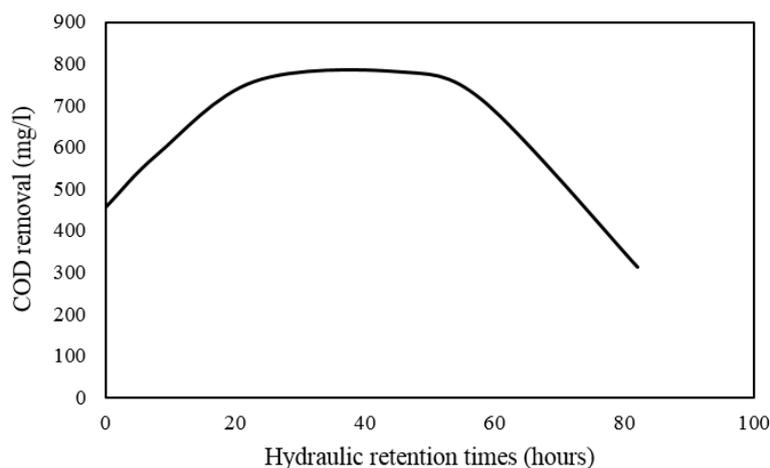
Figure 4. Effect of retention times on COD concentration.
