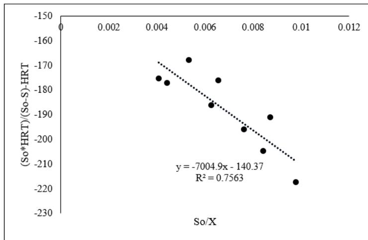
**Figure 9.** The second-order kinetic model for nitrate-N removal.
