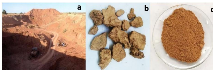
Figure 1. Outcrop of raw red clays from the Safi dam quarry and macroscopic appearance of the screened clay.
