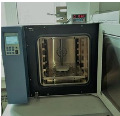
Figure 1. Thermo-furnace and weight-measuring device.
