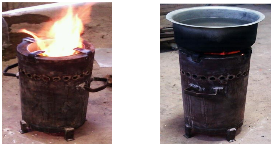
Figure 5. Flame of burning biomass and experimental work on IDBG cookstove.
