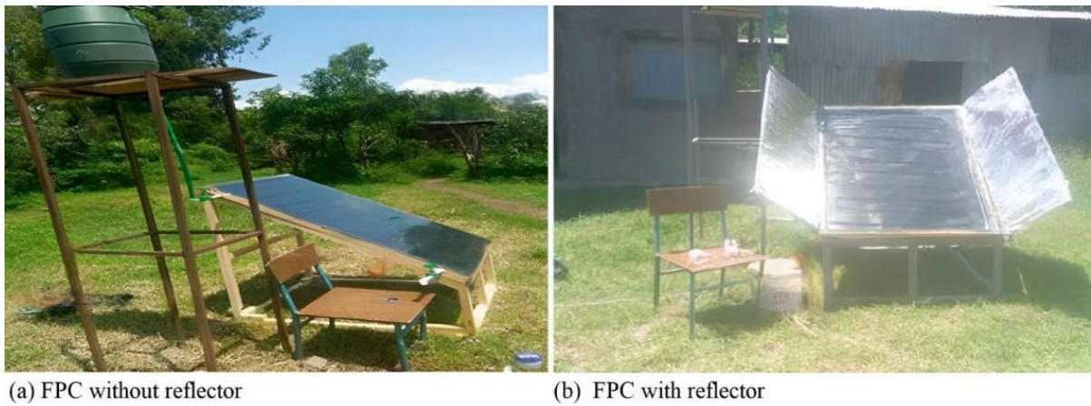
Figure 2. Experimental setup of milk pasteurization using FPC [54] .
