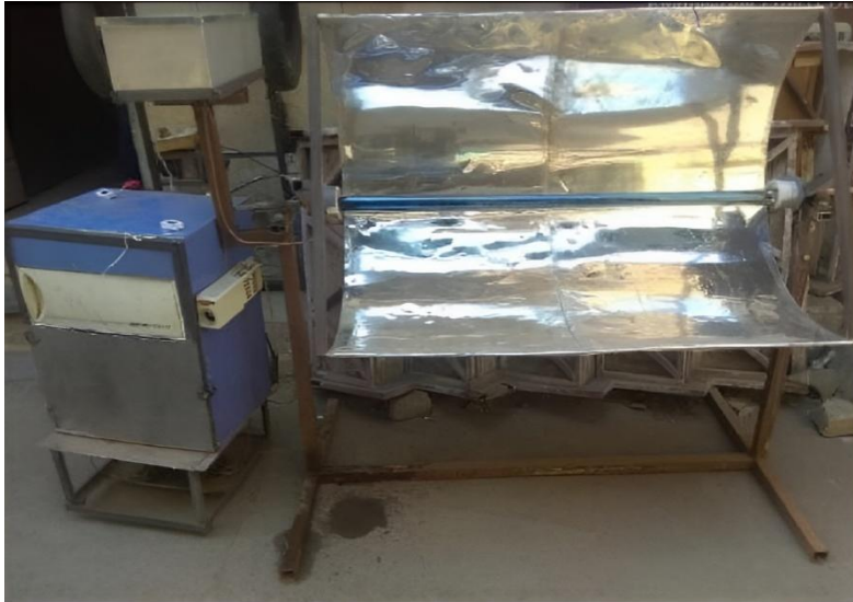
Figure 7. Milk pasteurization by parabolic concentrator with evacuated glass tube [2] .
