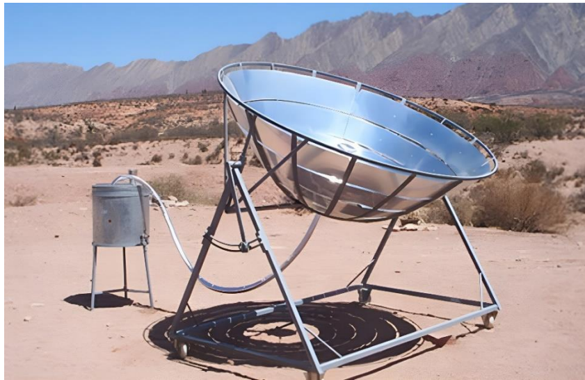
Figure 6. On-farm milk pasteurization system using Fresnel solar concentrator [67] .
