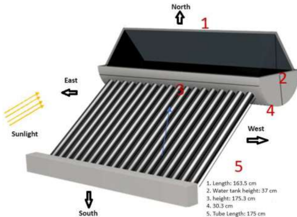
Figure 5. Schematic diagram of Semi-cylindrical tent shape SS coupled with ETC [38]
