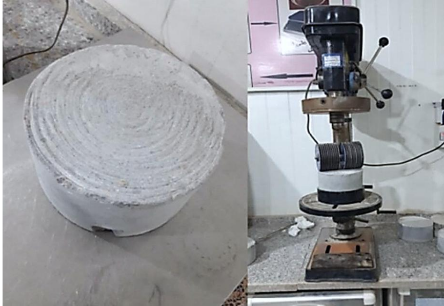
Figure 8. The rotary cutter device for evaluating the abrasion resistance and the electronic digital caliper.
