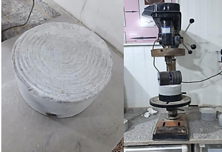
Figure 8. The rotary cutter device for evaluating the abrasion resistance and the electronic digital caliper.
