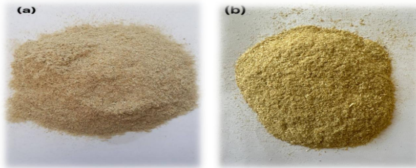
Figure 1. Samples of air dried and milled: (a) corn stalks and (b) wheat stalks.
