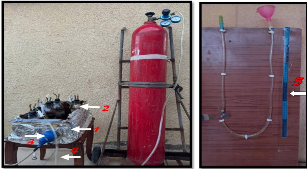
Figure 2. The experimental setup for the biogas generation system consists of the following basic components: (1) bath of water, (2) digester, (3) thermostat, (4) nitrogen purging rubber tube, and (5) manometer.
