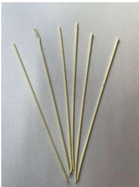
**Figure 2.** PP-g-C<sub>3</sub>N<sub>4</sub> filament samples.
