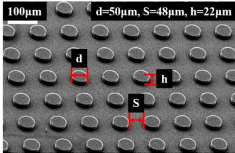
**Figure 1.** Micro/nano-textured surface image captured by a scanning electron microscope (SEM)
