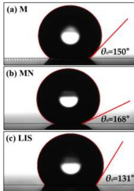
**Figure 2.** Measured contact angles on (a) Micro (M) (b) Micro/Nano-textured surfaces (MN) and (c) lubricant infused surfaces with Micro/Nano-textures (LIS).
