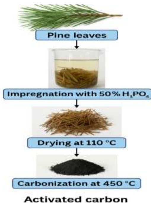
Figure 1. Preparation of pine leaves-based activated carbon by phosphoric acid
