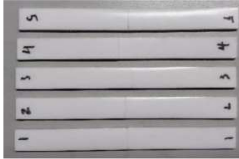
Figure 5. Fracture analysis of syntactic foam composite flexural testing.
