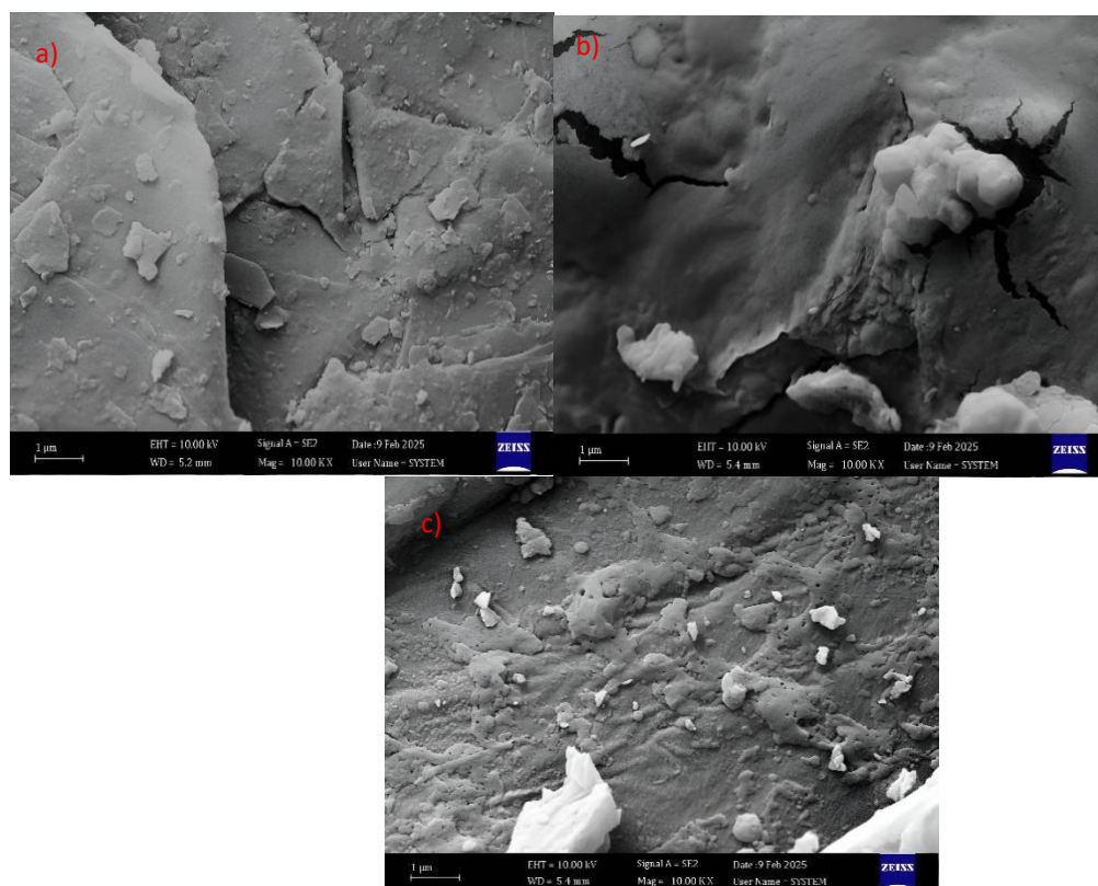
Figure 2. FESEM image of a) Activated carbon , b) activated carbon after methyl red (MR) , c) the activated carbon surface following methyl orange (MO)
