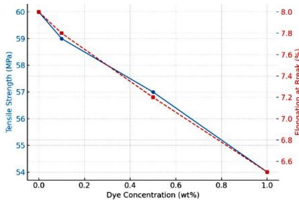
**Figure 4.** Influence of dye concentration on the mechanical properties of PLA. Increasing dye loading leads to reduced tensile strength and elongation at break, reflecting dye aggregation and microstructural disruptions within the polymer matrix.
