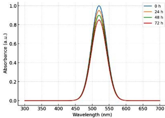
**Figure 3.** Thermal aging effect on Sudan Red-modified PLA specimens exposed at 80 °C for 72 h. Progressive reduction in absorbance intensity over time indicates gradual dye degradation, with ~15% reduction observed after 72 h.
