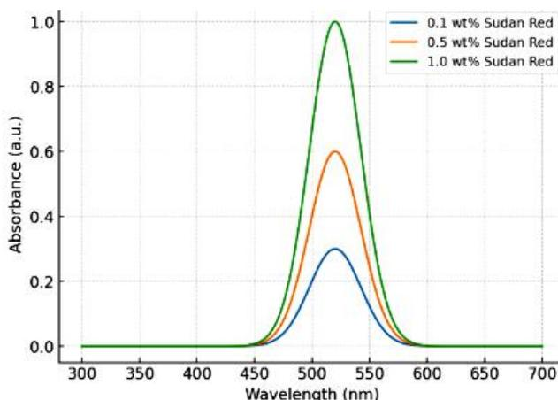
**Figure 1.** UV–V’s absorption spectra of Sudan Red-modified PLA filaments at different dye concentrations (0.1, 0.5, and 1.0 wt%). Increased absorbance intensity with higher concentrations confirms successful dye incorporation, while slight peak shifts indicate polymer–dye interactions.
