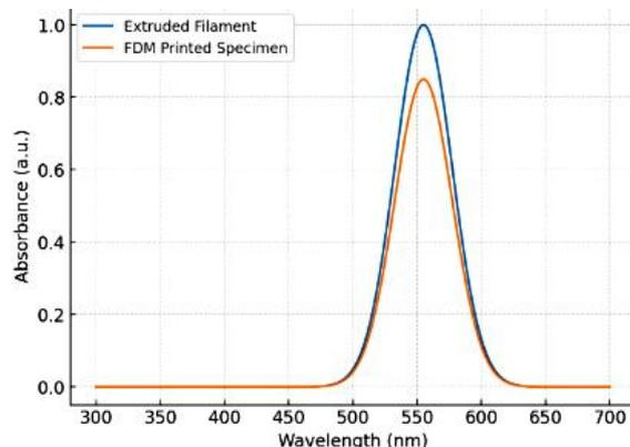
**Figure 2.** Comparison of UV–V’s spectra for Rhodamine B-modified PLA before and after FDM printing. The reduction in absorbance intensity (~15%) and peak broadening highlight partial thermal degradation and aggregation of dye molecules during layer-by-layer deposition.
