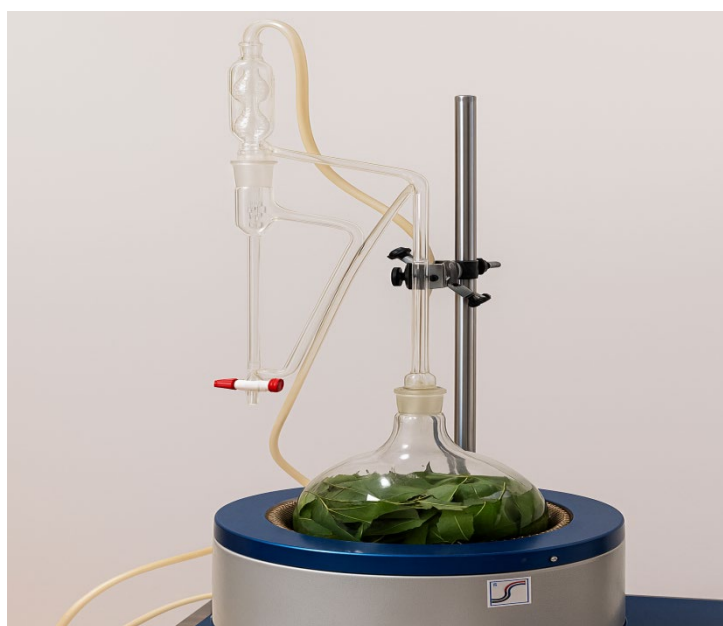
Figure 4. Hydrodistillation setup (Clevenger-type apparatus) used for essential-oil extraction under atmospheric pressure at 100 \pm 2 °C for 2–4 h.
