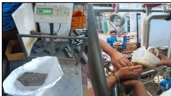
Figure 2. Medical plastic waste feed stock weighed and added in reactor.
