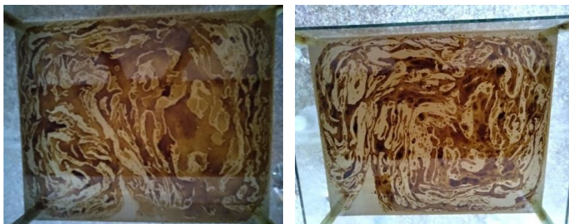
Figure 26. Oil slick disintegration after 1 and 24 hours of CMC-coated \text{Fe}_2\text{O}_3 NPs.
