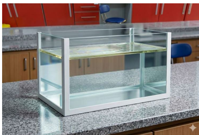
Figure 1. The laboratory system for removing oil slicks. Basin dimensions: 50 cm (length) × 40 cm (width) × 30 cm (height). 3 .
