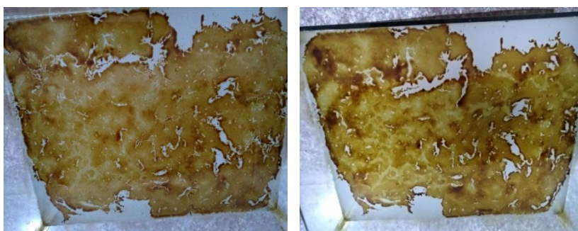
Figure 24. Oil slick disintegration after 6 and 24 hours of CMC-coated \text{Al}_2\text{O}_3 NPs.
