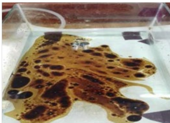
Figure 22. The contaminated oil slick on the basin water surface.
