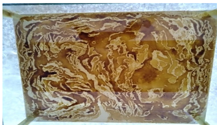
Figure 28. Oil slick disintegration after 24 hours of CMC-coated \text{Fe}_2\text{O}_3 NPs.
