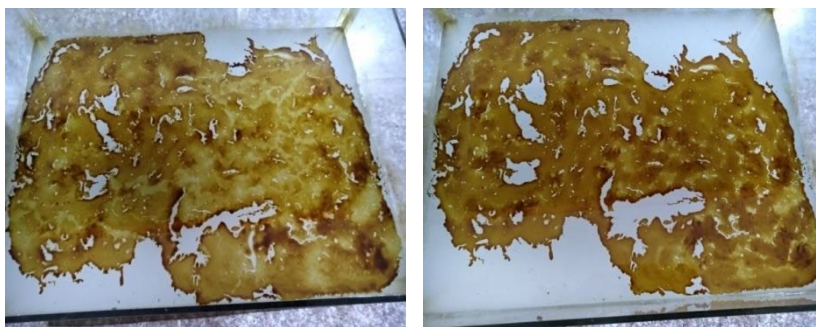
Figure 29. Oil slick disintegration after 1 and 6 hours of CMC-coated \text{Al}_2\text{O}_3 NPs.
