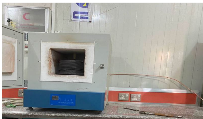
Figure 3. Photograph of the experimental setup used for the activation process under nitrogen atmosphere.
