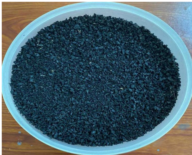
Figure 1. shows a photograph of the raw waste tire crumb rubber before any thermal or chemical treatment, illustrating the irregular particle morphology and size distribution of the starting material.
