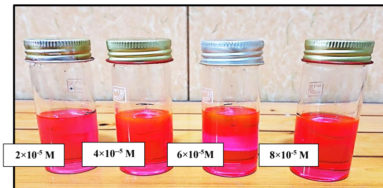
Figure 2. Organic laser dyes mixture with different concentrations.
