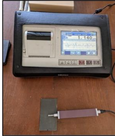
Figure 4. Mitutoyo SJ-310 contact stylus profilometer employed for surface roughness measurement in accordance with ISO 4287/4288.
