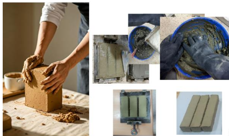
Figure 4. Photographs of prepared clay-based composite specimens reinforced with Cynodon dactylon fibres.
