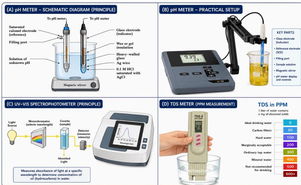
Figure 3. Laboratory instruments utilized for the analysis of water quality: (A–B) pH meter and its principle of measurement, (C) oil concentration analysis using a UV–Vis spectrophotometers, and (D) meter for measuring dissolved solid in ppm by TDS [19,20] .
